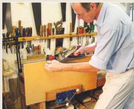
▲ Pic.4 Tidy up furry edges by chamfering freehand; this is good practice at freehand work
